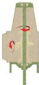
*Mixer shaft is supported independently. It is mounted in separate bearings that carry only the mixer shaft loads.*
