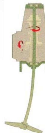
*Shaft flexure is isolated from gears. The drawing shows in exaggerated fashion how the mixer shaft can flex dramatically in the hollow quill with no effect on the drive, gearing is protected to add years of service.*
