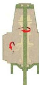
*Mixer shaft is flexibly coupled to the quill. A torsionally resilient coupling transmits power from quill to mixer shaft, through a steel taper grid member that freely adjusts to shaft flexure.*
