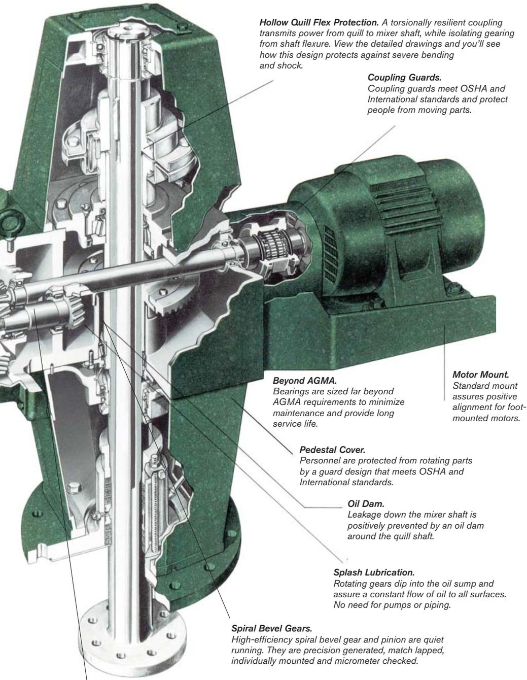
**Hollow Quill Flex Protection.** A torsionally resilient coupling transmits power from quill to mixer shaft, while isolating gearing from shaft flexure. View the detailed drawings and you'll see how this design protects against severe bending and shock.
