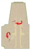
*Hollow quill assembly with bevel gear is mounted in its own heavy-duty bearings.*
